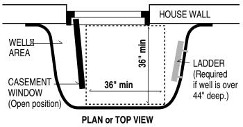
Note: Centering a window well at the window might not give you the required minimum 36 inches. Measure carefully!
