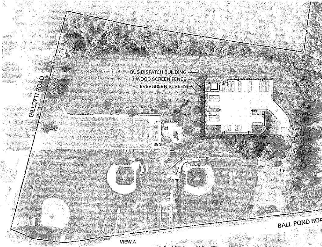
Conceptual plan rendering indicating additional screening on the northern, southern, and eastern sides of the school bus lot.
