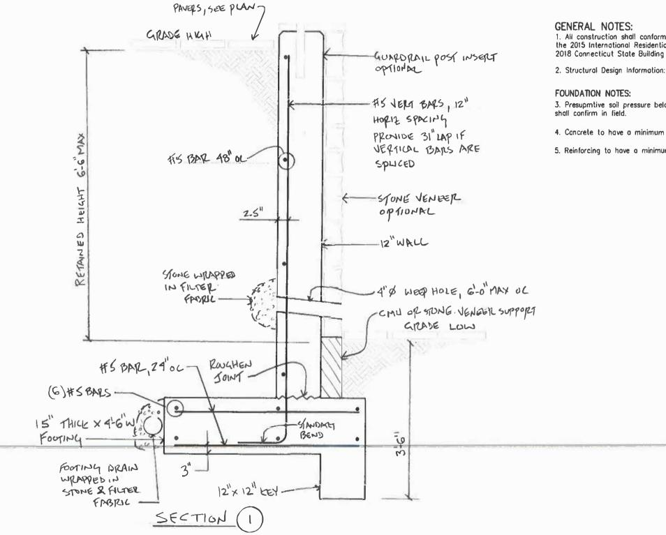
**GENERAL NOTES:** 1. All construction shall conform the minimum requirements of the 2015 International Residential Code as modified by the 2018 Connecticut State Building Code.
