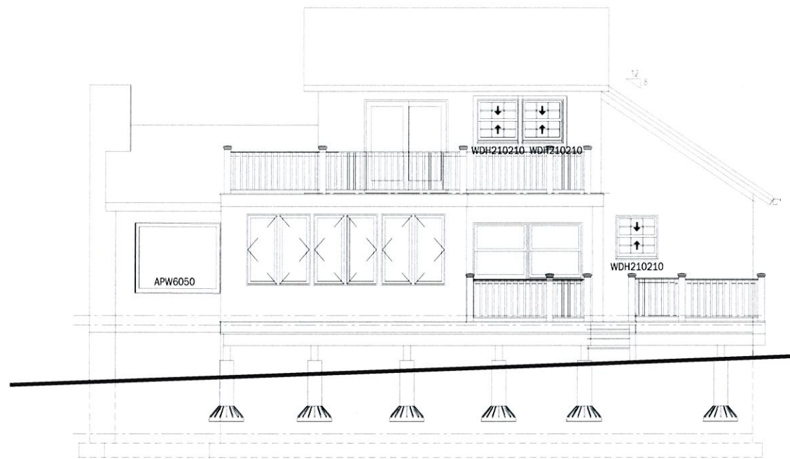
PROPOSED REAR (EAST) ELEVATION SCALE: 1/4" = 1'-0"
