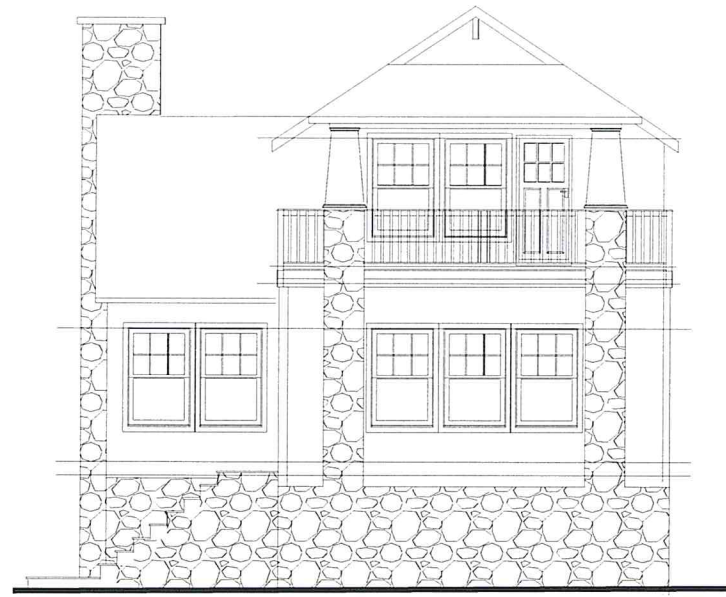
PROPOSED FRONT (EAST) ELEVATION SCALE: 1/4" = 1'-0"
