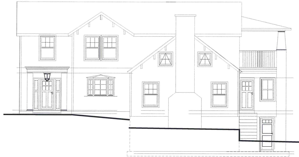
PROPOSED SIDE (SOUTH) ELEVATION SCALE: 1/4" = 1'-0"
