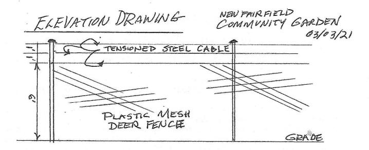
1. STEEL CORNER POSTS TO BE SET INTO METAL SLEEVES
